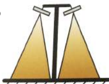
Wall-mounted (Tunnel lighting)
