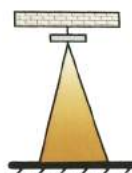
Suspend-mounted (Baylight High / Low)
