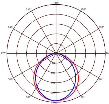
C00 Plane beam angle(50%):109.5(DEG) C90 Plane beam angle(50%):99.1(DEG)
